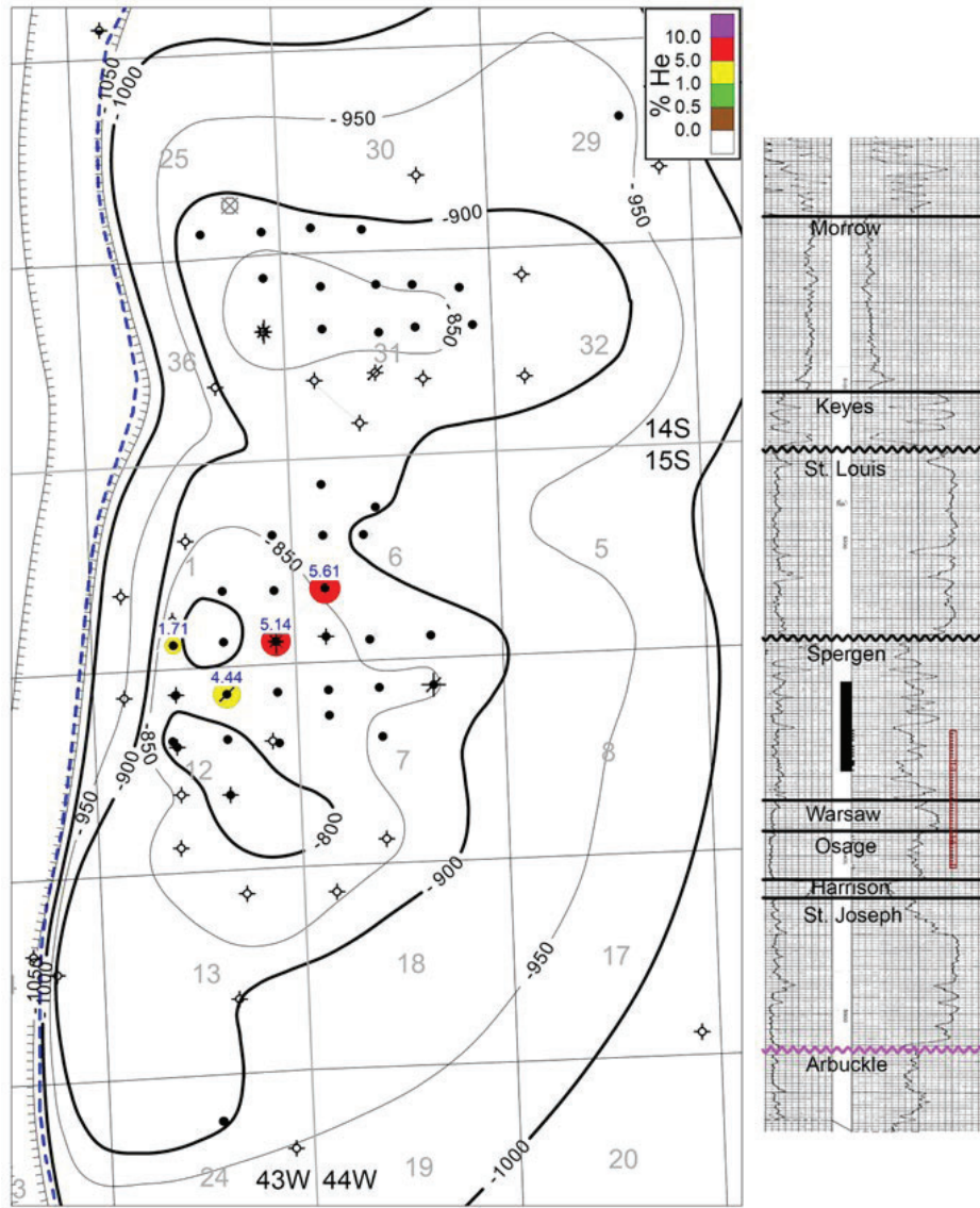
Figure 9. LEFT: Structure map, Ladder Creek-Spergen Field contoured on top of Mississippian Saint Louis formation (c.i. 50 ft., 15 m). Blue numbers are reported percentages of helium. Helium plant is in Section 25, T14S, R43W. RIGHT: Type neutron log. Helium production is from the stratigraphic interval indicated by the black rectangle.
